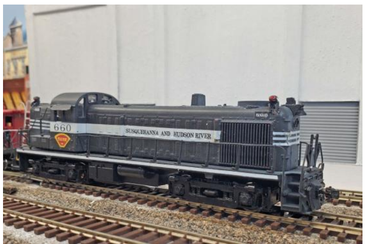
Photo 10. S&HR 660, an Alco RS-3 unit, displays the family look of the Alco road switchers on the S&HR. Bell mounted high on the front of the engine with bug-eye classification lights on each corner.
