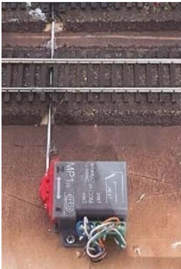
Fig. 9. Left: Surface mounted MP1 using an aluminum tube to route the music wire actuator rod. Right: The MP1 is small enough to be hidden within a building on my layout.
