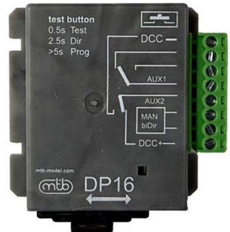
Fig. 7. The DP 16 is designed to provide dual control by DCC and local control via push button or toggle switch.
