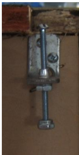
Fig. 4. Limit switch stop adjustment.
