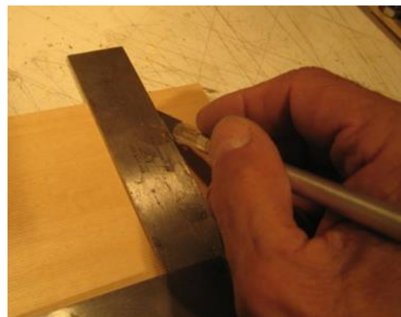
Fig. 9. Position the square to prevent the knife from straying onto the good wall section.
