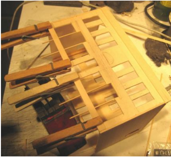
Fig. 16. Initial framing for the windows and doors.
