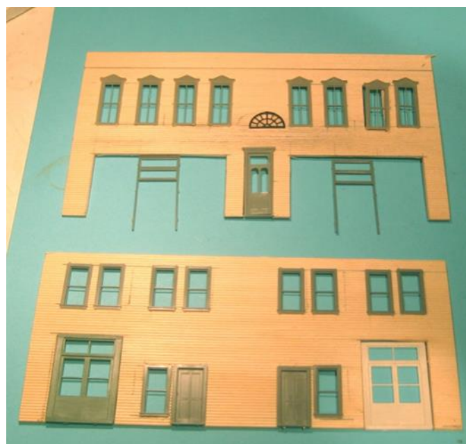
Fig. 12. Test fitting the doors and windows.
