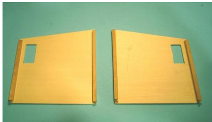
Fig. 13. The side walls need to be mirror images.
