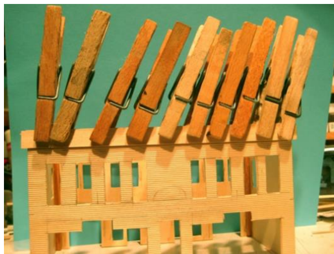
Fig. 15. Clothespins are inexpensive, readily available clamps.
