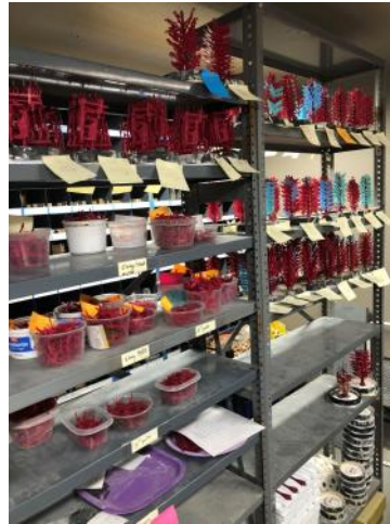
Left: The red items are wax patterns still on "runners." These are used to make the molds in the lost-wax brass casting process. Right: The autoclave used to melt and force the wax out of the mold, which will eventually be filled with molten brass.
