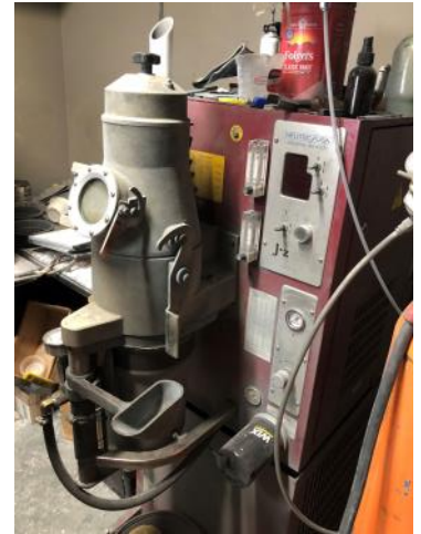
Left: The red items are wax patterns still on "runners." These are used to make the molds in the lost-wax brass casting process. Right: The autoclave used to melt and force the wax out of the mold, which will eventually be filled with molten brass.
