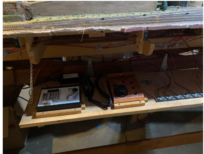
Digitrax DCS51 command station and Atlas switches.
