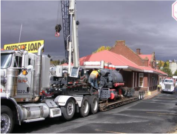
Strapping down locomotive
