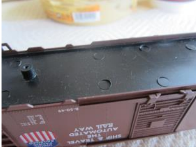
Mold release points on the car floor.
