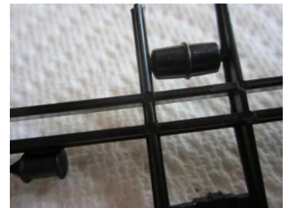
Mold release points along the frame.
