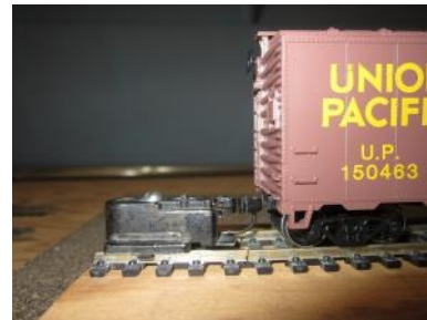
The new Kadee coupler height gauge is insulated.
