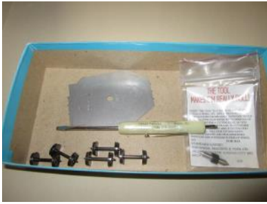
NMRA gauge, Truck Tuner, and screw driver along with some new metal wheels ready for replacement.
