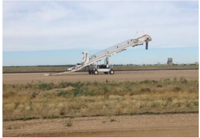
Self-propelled sand conveyor placed under a hopper car lifts sand into an adjacent truck.
